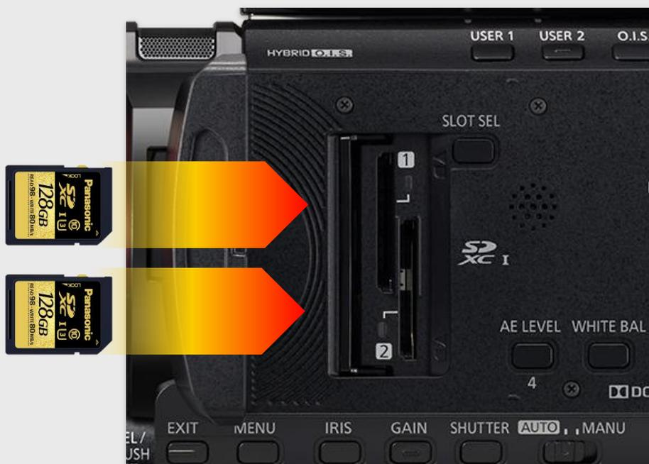
\* Maximum file size that can be recorded over multiple SD cards is 96 GB. Recording will not stop even when the data size exceeds 96 GB.
