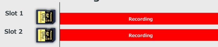
Identical data is recorded onto cards in both slots in this highly redundant recording mode.
