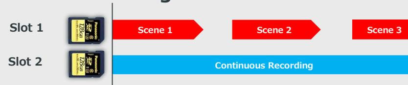
Records ordinary Rec Start/Stop-controlled data in Slot 1, and records all data, even when the camcorder is stopped, in Slot 2.
