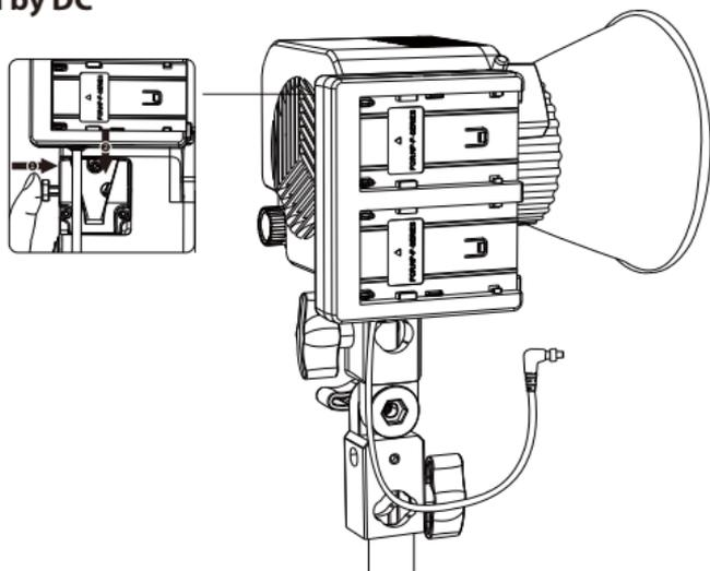
*\*The batteries are not included. Please press the spring-loaded lock button on the battery plate to remove the power cord. Do not pull it out forcibly.*
