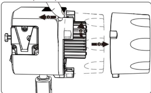
*\* Notice: Always remove the protection cover prior to turning on the light. Always re-install the cover when packing it away.*
